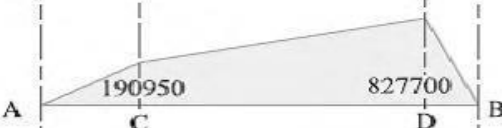
(f) Horizontal B.M. diagram.
