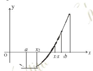
if f(x) = 0, then  $x_1$  is the root of equation f(x) = 0. Otherwise the root lies between a and  $x_1$  or  $x_1$  and  $x_1$  and  $x_2$  or  $x_1$  and  $x_2$  or  $x_2$  and  $x_2$  or  $x_2$  and continue the process until the root is found to desired accuracy.
