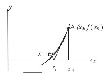
In this method, instead of taking two initial rough approximations to the root x = a as in the previous two methods, a single rough approximation  $x_0$  to the root is taken. Then we use the following formula, known as Newton-Raphson formula or Newton iteration formula, to get the successive approximations.
