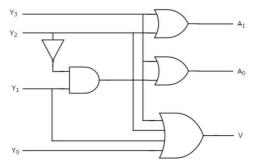
The above circuit diagram contains two 2-input OR gates, one 4-input OR gate, one 2input AND gate & an inverter. Here AND gate & inverter combination are used for producing a valid code at the outputs, even when multiple inputs are equal to '1' at the same time. Hence, this circuit encodes the four inputs with two bits based on the **priority** assigned to each input.
