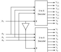
The parallel inputs  $A_2$ ,  $A_1$  &  $A_0$  are applied to each 3 to 8 decoder. The complement of input, A3 is connected to Enable, E of lower 3 to 8 decoder in order to get the outputs,  $Y_7$  to  $Y_0$ . These are the **lower eight min terms**. The input,  $A_3$  is directly connected to Enable, E of upper 3 to 8 decoder in order to get the outputs,  $Y_{15}$  to  $Y_8$ . These are the **higher eight min terms**.
