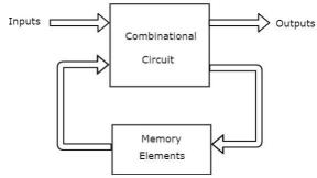
This sequential circuit contains a set of inputs and outputss. The outputss of sequential circuit depends not only on the combination of present inputs but also on the previous outputss. Previous output is nothing but the **present state**. Therefore, sequential circuits contain combinational circuits along with memory storage elements. Some sequential circuits may not contain combinational circuits, but only memory elements.
