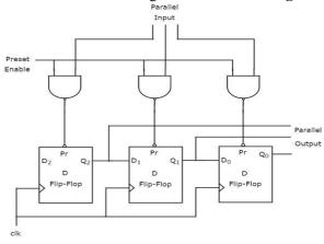
This circuit consists of three D flip-flops, which are cascaded. That means, output of one D flip-flop is connected as the input of next D flip-flop. All these flip-flops are synchronous with each other since, the same clock signal is applied to each one.
