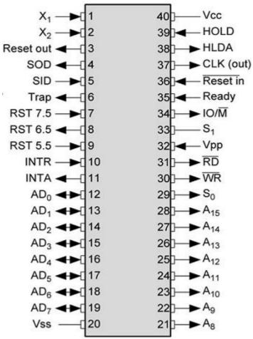
The pins of a 8085 microprocessor can be classified into seven groups – Address bus
