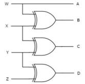
Since the outputs depend only on the present inputs, this 4-bit Binary code to Gray code converter is a combinational circuit. Similarly, you can implement other code converters.
