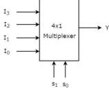
One of these 4 inputs will be connected to the output based on the combination of inputs present at these two selection lines. **Truth table** of 4x1 Multiplexer is shown below.
