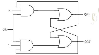
This circuit has two inputs J & K and two outputs Qtt &Qtt'. The operation of JK flip-flop is similar to SR flip-flop. Here, we considered the inputs of SR flip-flop as S = J Qt' and R = KQt in order to utilize the modified SR flip-flop for 4 combinations of inputs.
