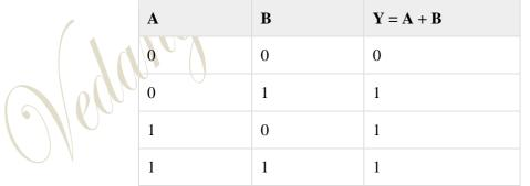
Here A, B are the inputs and Y is the output of two input OR gate. If both inputs are '0', then only the output, Y is '0'. For remaining combinations of inputs, the output, Y is '1'.
