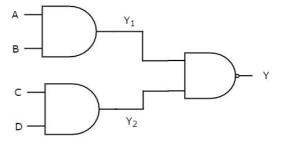
Previously, we got the outputs of first level logic gates as Y1=AB and Y2=CD
