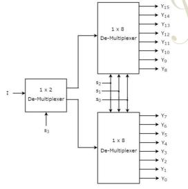
The common selection lines  $s_2$ ,  $s_1 \& s_0$  are applied to both 1x8 De-Multiplexers. The outputs of upper 1x8 De-Multiplexer are  $Y_{15}$  to  $Y_8$  and the outputs of lower 1x8 DeMultiplexer are  $Y_7$  to  $Y_0$ .
