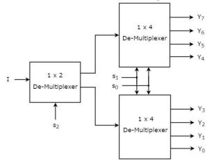
The common selection lines,  $s_1 \& s_0$  are applied to both 1x4 De-Multiplexers. The outputs of upper 1x4 De-Multiplexer are  $Y_7$  to  $Y_4$  and the outputs of lower 1x4 De-Multiplexer are  $Y_3$  to  $Y_0$ .
