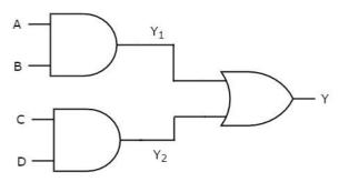
Previously, we got the outputs of first level logic gates as Y1=AB and Y2=CD.
