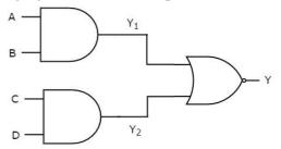
We know the outputs of first level logic gates as Y1=AB and Y2=CD
