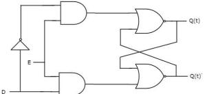
This circuit has single input D and two outputs Qt & Qt'. D Latch is obtained from SR Latch by placing an inverter between S amp;& R inputs and connect D input to S. That means we eliminated the combinations of S & R are of same value.
