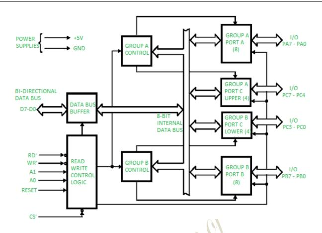
It consists of 40 pins and operates in +5V regulated power supply. Port C is further divided into two 4-bit ports i.e. port C lower and port C upper and port C can work in either BSR (bit set rest) mode or in mode 0 of input-output mode of 8255. Port B can work in either mode 0 or in mode 1 of input-output mode. Port A can work either in mode 0, mode 1 or mode 2 of input-output mode.
