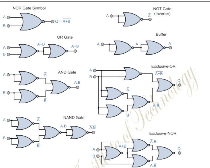
Thus ALL other logic gate functions can be created using only NOR gates making it also a universal logic gate.
