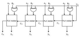
If initial carry,  $C_0$  is zero, then each full adder gets the normal bits of binary numbers A & B. So, the 4-bit binary adder / subtractor produces an output, which is the **addition of two binary numbers** A & B.
