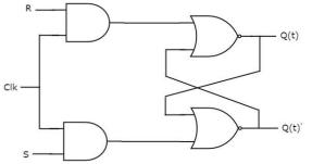
This circuit has two inputs S & R and two outputs Qt & Qt'. The operation of SR flip is similar to SR Latch. But, this flip-flop affects the outputs only when positive transition of the clock signal is applied instead of active enable. The following table shows the **state table** of SR flip-flop.
