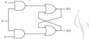
This circuit has two inputs S & R and two outputs Qt & Qt'. The **upper NOR gate** has two inputs R &complement of present state, Qt' and produces next state, Qt+1 when enable, E is '1'.
