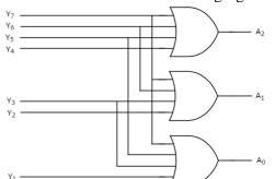
The above circuit diagram contains three 4-input OR gates. These OR gates encode the eight inputs with three bits. Drawbacks of Encoder
