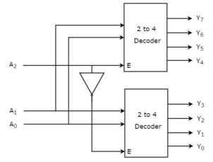
The parallel inputs  $A_1 \& A_0$  are applied to each 2 to 4 decoder. The complement of input  $A_2$  is connected to Enable, E of lower 2 to 4 decoder in order to get the outputs,  $Y_3$  to  $Y_0$ . These are the **lower four min terms**. The input,  $A_2$  is directly connected to Enable, E of upper 2 to 4 decoder in order to get the outputs,  $Y_7$  to  $Y_4$ . These are the **higher four min terms**.
